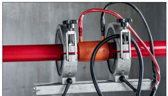
Fig. 03-14 Secure the welding cable by looping a section of it to prevent it being pulled off inadvertently.
