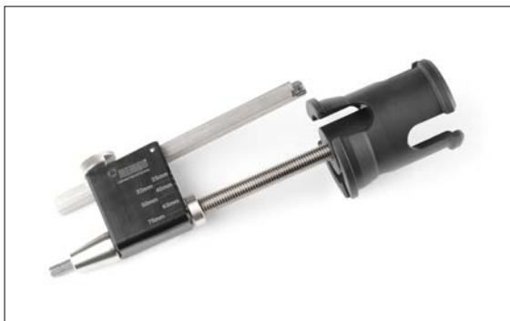
Fig. 03-3a A rotary pipe scraper must be used to scrape the pipe ends. The figure shows the “SMARTFUSE DUO 25-75”. A hand crank or cordless screwdriver can be used to drive it.
