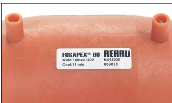
Fig. 03-17 The joint must not be subjected to any loads during the cooling down time specified on the fitting. For pipes under tension (e.g. pipe coils), observe the extended cooling down time in Tab. 03-4. Only then may the pipe retaining clamps be removed.
