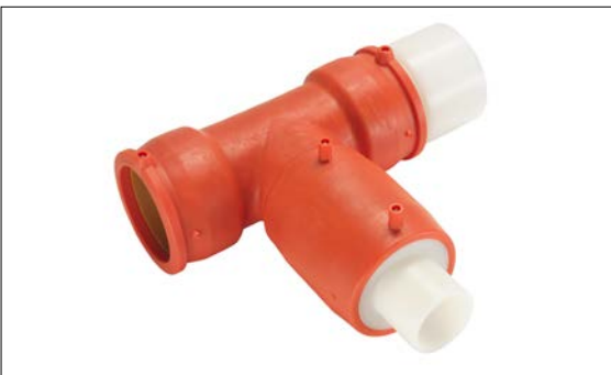
Fig. 03-33 When welding combined components, you must comply with the cooling down times between two connection welds. The following welding sequence has proven effective: ▪ For a T-piece, connecting passage before outlet ▪ For reducers, small before large
