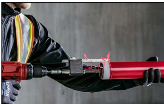
Fig. 03-4 Drive the rotary scraper at a consistent high speed. A single continuous swarf will be created. If this is not the case, check the cutting blade and adjust the speed.
