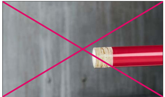
Fig. 03-25 The welding area must not be wet or soiled. If carrying out the work outside, you may need to set up a tent.
