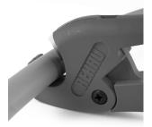
Use an approved plastic pipe cutter to cut the pipe to the desired length.
