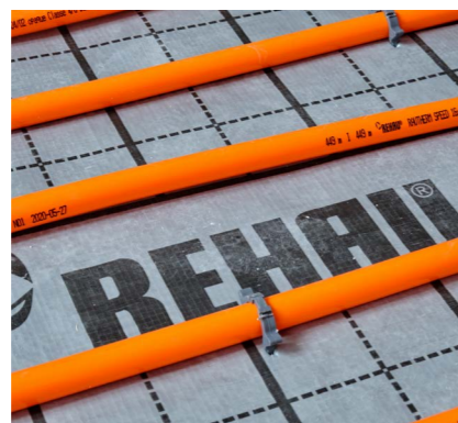
Tacker staples Uses staples to attach the pipe to a grid pattern membrane. Ideal for large areas where liquid screed is used.
