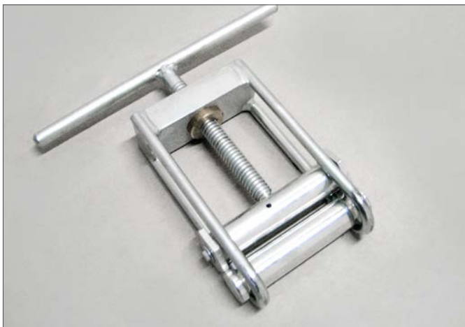
Fig. 1 Example squeeze-off tools for various pipe dimensions. Mechanical and/or hydraulic/mechanical
