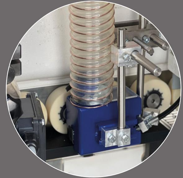
The application unit is connected to the existing machine exhaust. The switching and workpiece detection is carried out via the known RIEPE® electronics or via integration into the machines PLC by your machine manufacturer.
