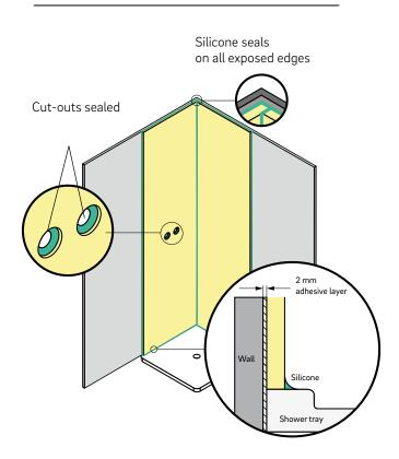
To seal the outer and abutting edges, REHAU recommends silicone grouting across all exposed edges to prevent the ingress of moisture, dirt, waterlogging and mold.
