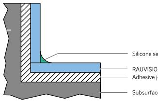
Silicone sealing joint (only necessary for applications exposed to water)
