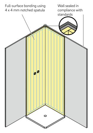
Due to joints and connection points on surfaces that are directly exposed to moisture, this requires the installation of additional sealing (sealing membranes or liquid sealants) under the wall covering. The stress classes for moisture exposure as defined in DIN 18531 must be taken into account.
