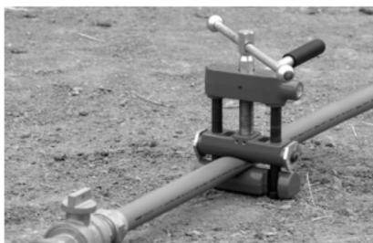
Fig. 12: Pipe in squeeze-off tool
