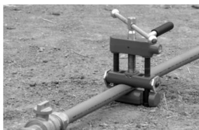
Fig. 12: Pipe in squeeze-off tool
