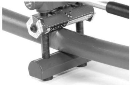
*Fig. 15: Re-rounding pipe*
