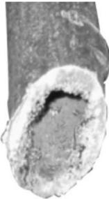
Fig. 2: Corrosion build-up in metal pipes
