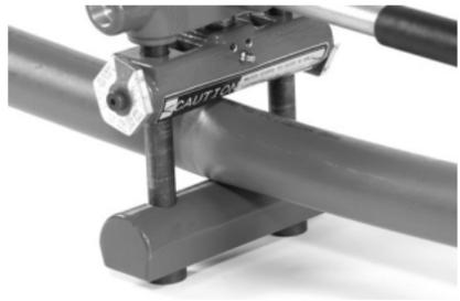
*Fig. 15: Re-rounding pipe*
