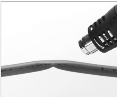
Fig. 11: Repair kinks using hot air
