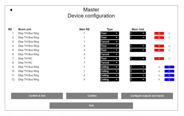
In this case, the fan coil is automatically assigned to the room unit, which is paired to this zone.
