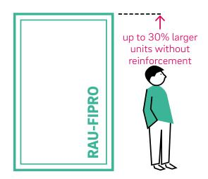
Fully self-reinforced sash, with RAU-FIPRO extending right into the fusion welded corners, provides excellent stability and torsional rigidity making it possible to build larger windows – without the need for metal reinforcement.
