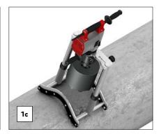
1. The drill is to be secured using appropriate equipment between 270° and 90° (e.g. using a drilling stand, ground pegs, suction cup or tension belts).
