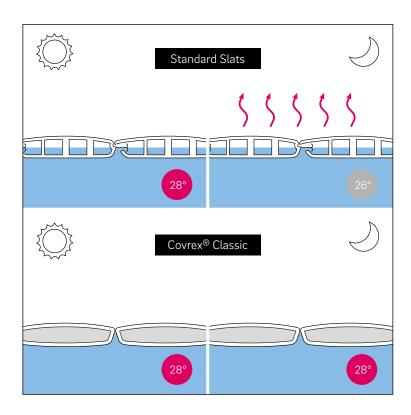
The COVREX® by REHAU minimizes the risks of algae development and dirt accumulation through its design by reducing the number of dead zone areas such as slates locking areas. In addition the foaming avoids the use of endcaps avoiding the risk of water ingress and offering a better durability in use.
