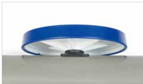
Figure 29: Bottom view of installed disc aerator (disc aerator lower rim touches top of the grommet)
