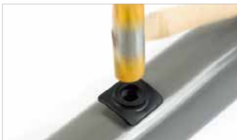
Figure 28: Grommet installation into a 32 mm hole using a rubber mallet
