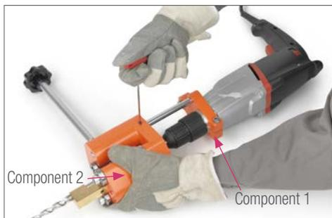
14. Turn the guide rollers anti-clockwise using toggle screw. Insert the milling fixture into the saddle outlet vertically and drill into the main pipe during this process. Tighten the toggle screws whilst the drill is running until the guide rollers are free of clearance at the saddle outlet.
