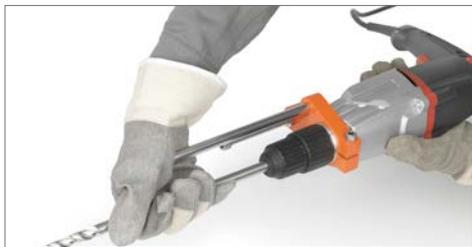
13. Insert Component 1 incl. drill machine into Component 2 up to the adjusting screw (distance approx. 9 cm) and secure on both sides with a grub screw M6.
