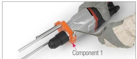
12. Insert the milling drill into the drill machine and lock.
