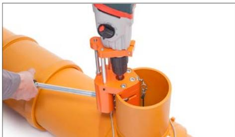
17. Move the guide rollers back using the toggle screw. Take out the milling fixture and the milled out section and remove the clamping rope.
