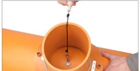
11. Attach Component 1 to the collar of the drill machine using a 6 mm external hexagon socket wrench.
