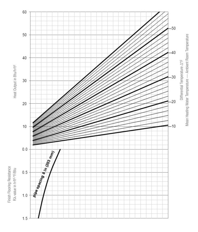
Figure 7: Talon-Up (No Heat Transfer Plates) With 1/2 in. RAUPEX (Subfloor 3/4 in [18 mm] Plywood)
