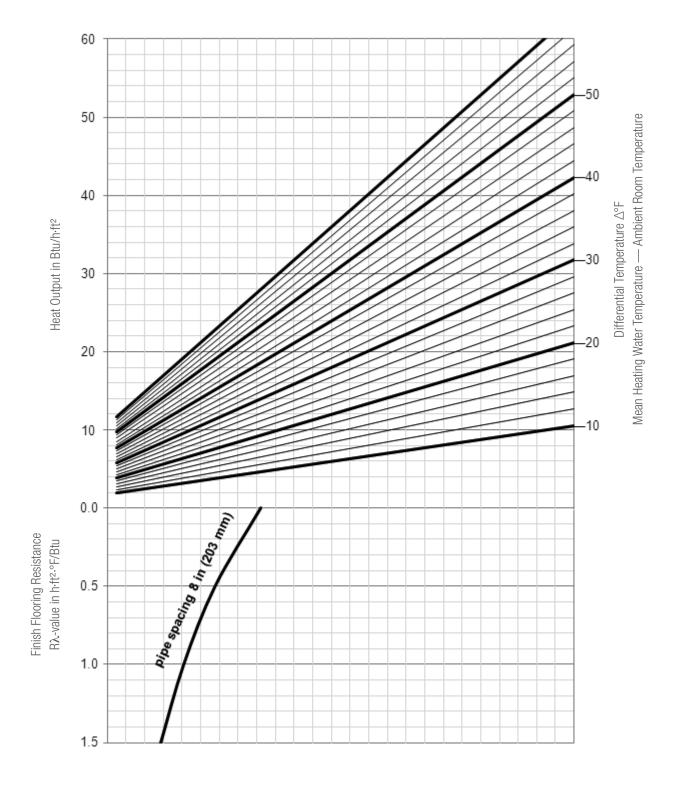
Figure 5: Heavy Gauge Heat Transfer Plates With 1/2 in. RAUPEX (Subfloor 3/4 in [18 mm] Plywood)
