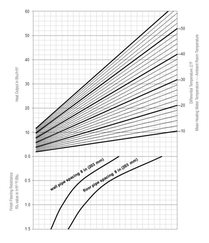
Figure 3: RAUBOARD Heat Transfer Panels With 10.1 mm RAUPEX
