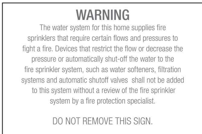
Fig. 6.1: Warning sign for main water shut-off
