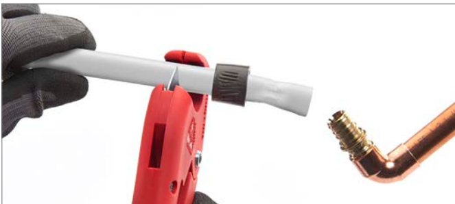
Fig. 5.11: Cut off 3 in. of pipe from end prior to making new joint
