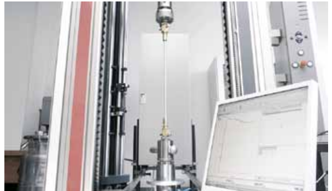
Proceeding a tension test with compression sleeve joint
