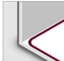
Fig. 4-7 groove mounted (milled)
