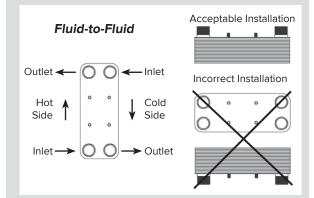
**Steam** applications - unit should be installed in a vertical position to ensure the condensate drains from the heat exchanger.
