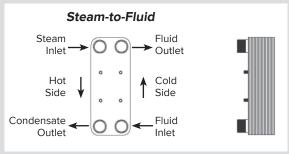
**Refrigeration** applications – Heat exchanger must be installed in a VERTICAL position.
