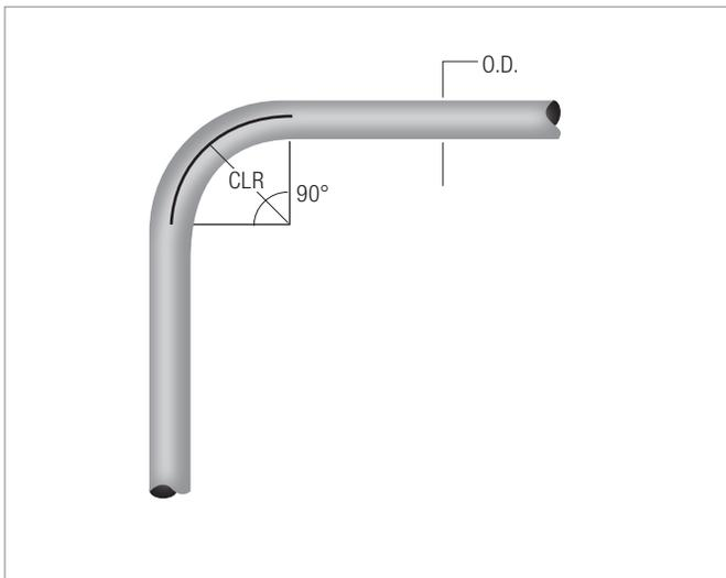
Fig. 4.3: Centerline radius (CLR) of RAUPEX pipe
