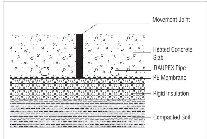
Fig. 5.2: Movement joint
