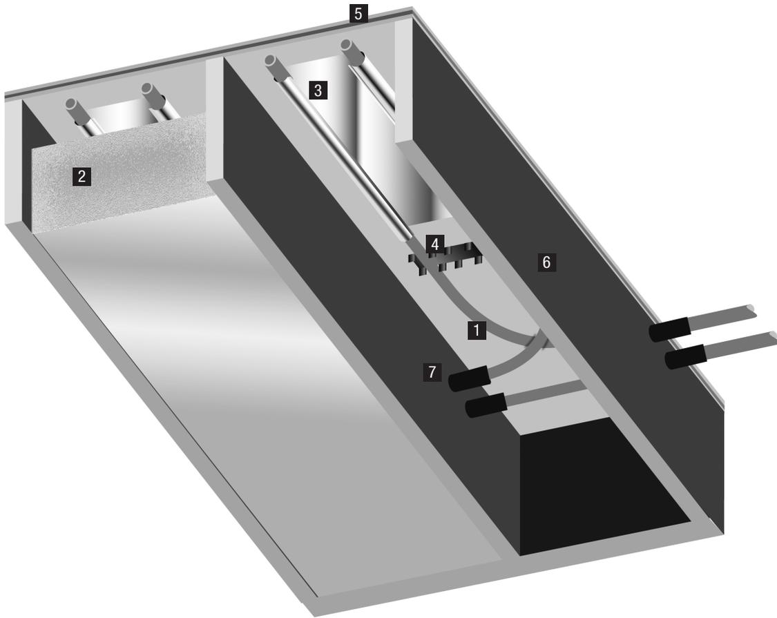
**1 RAUPEX Pipe** - Snaps securely into the RAUPLATE channels without adhesives or fasteners. When transitioning from the joist penetration to the heat transfer plates, criss-crossing the pipes increases the bending radius and makes them easier to install.
