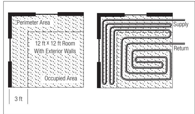
Fig 6.4: Overpour with perimeter and occupied areas using one circuit
