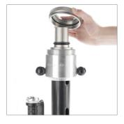
In confined assembly situations, use an Allen key to release and turn the tool handle.
