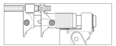
6. Bring selector button into sliding position (upper position of button).
