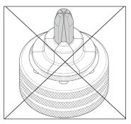
Make sure fitting is correctly seated in tool. Applying the tool to the wrong fitting collar will over-compress the joint.
