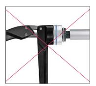
Before operating the tool, the correct fit and the compression effect of the expander bit in the clamping jaws must be checked. The expander bit must sit tightly in the clamping jaws and may not fall out.
