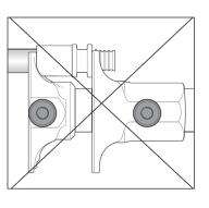
If using an expander bit, make sure the bit is in the correct position (completely inserted into the jaw) before starting tool and ensure lock screw is tightened.
