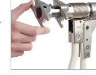
3. The clamping jaws are brought into the correct position by turning the tool cylinder.
