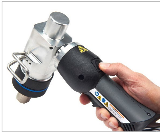
Fig. 10 Press release button to release hydraulic pressure
