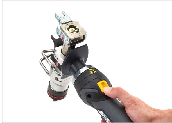
Fig. 2 Press release button to release hydraulic pressure
