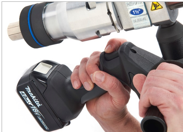
Fig. 5 Use only index finger to trigger tool
