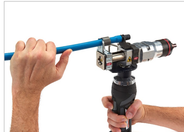
Fig. 4 Proper hand positioning during compression
