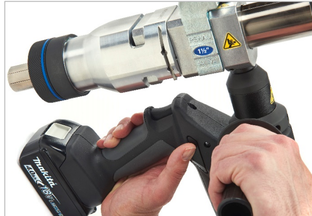
Fig. 6 Press release button to release hydraulic pressure
