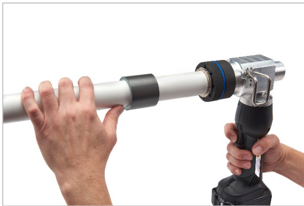
Fig. 11 Proper hand positioning during expansion
