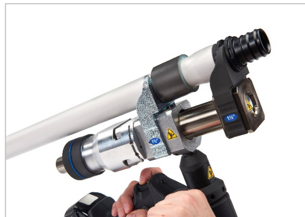
Fig. 8 Proper hand positioning during compression
