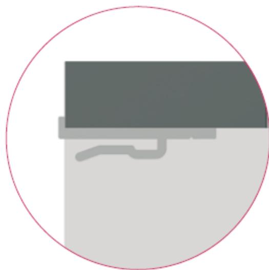
**Step 3:** To complete door installation, insert the cover profile into the mounting piece clip.
