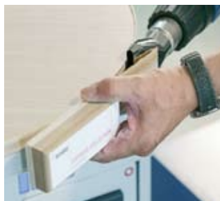
3 Polishing Felt and Heat Gun Finishes the joint adhesion
