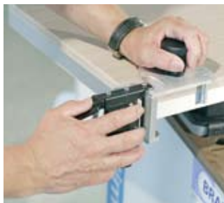
1 Guillotine End Trimmer Trims the edgeband ends with precision
