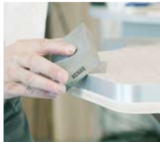
8 Sponge Sanding Block Deflashes edges that cannot be radiused
