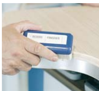
6 Finisher Sands edges to eliminate processing traces
