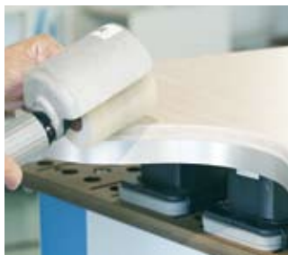
7 Polisher with Flap Wheel Smooths and rounds edges after trimming
