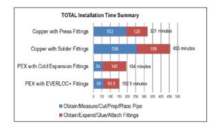
EVERLOC+ was fastest in the hallway using large diameter fittings (1 1/4 in. and above):
