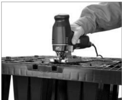
*Separation of a basic element along the cutting mark*
