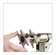
4. Exchange of clamping jaws should always be carried out in the starting position (maximum deflection of the tool lever).
