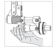
Check for fit (clamping) before use to avoid falling out.
