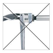
Before operating the tool, the correct fit and the compression effect of the expander bit in the clamping jaws must be checked. The expander bit must sit tightly in the clamping jaws and may not fall out.
