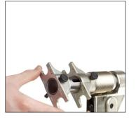
2. Insert the short pin into the long clamping jaw and the long pin into the short clamping jaw.
