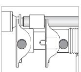
Always insert expanding tool into pipe as far as it will go.
