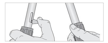
9. Press lever **again** until safety catch is released. Then move lever up 90° to return tool to starting position.
