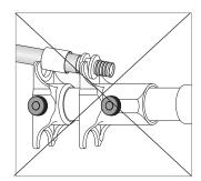
Never use damaged expander head as this will damage the pipe. Replacements are available from your local REHAU representative.
