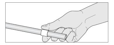
3. Expand pipe using expander or expander bit. Rotate 30° and repeat. The minimum distance between expander head and compression-sleeve must be one compression-sleeve length.
