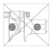
If using an expander bit, make sure the bit is in the correct position (completely inserted into the jaw) before starting tool and ensure lock screw is tightened.
