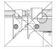
Regularly grease the expanding tool taper using tube of lubricant supplied with the tool.
