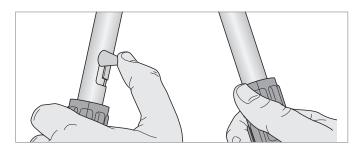
7. Activate lever to push compression sleeve up to fitting collar.
