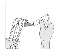
**Note:** Do not apply any grease to the surface of the expanding segments that come in contact with the pipe.
