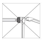
Transition fittings with a large external diameter must be laid and compressed on the "free side."
