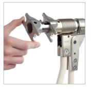
2. Insert the short pin into the long clamping jaw and the long pin into the short clamping jaw.
