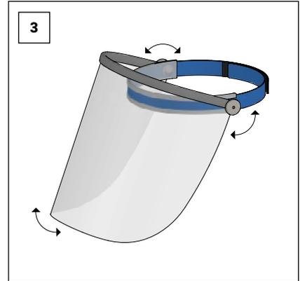
Slightly loosen the fixing screws, adjust the angle of the umbrella and pull the fixing screws tight again.
