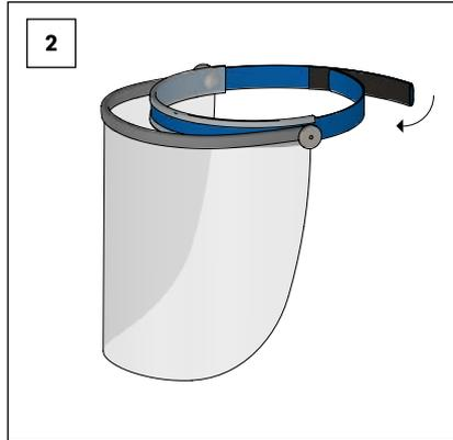
Put Face Shield on the head and fasten with velcro close tightly.
