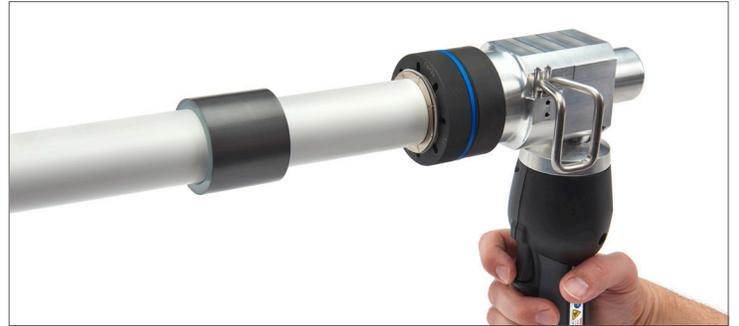
7. To release the hydraulic pressure and return the tool to its starting position, press the release button.
