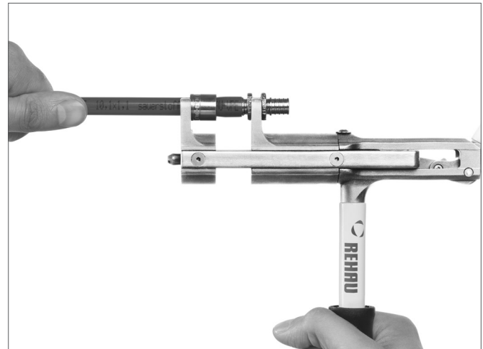
Fig. 20: Compressing fitting with K10 tool
