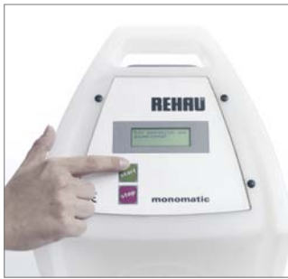
Fig. 50 12. Pressing the start button a second time will initiate the welding process.
