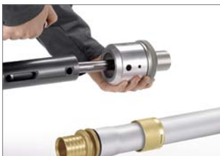
Fig. 21 5. Remove the expansion unit from the tool.
