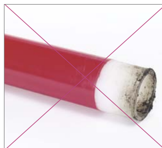
Fig. 120 The welding zone must be dry and dirt-free.
