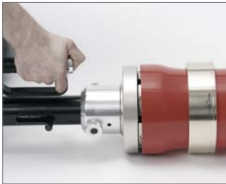
Fig. 29 4. The fitting insertion time in the pipe can be influenced by holding the expansion pressure with expansion head fully open (expansion process end position).
