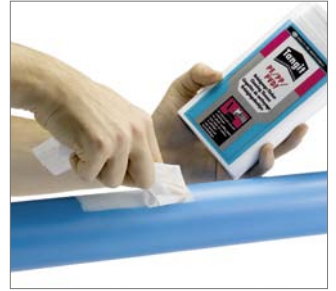
Fig. 55 3. The scraping area must be free of dirt and oil. Clean the area with an adequate amount of Tangit cleaner, and subsequently allow the cleaning agent to completely evaporate.
