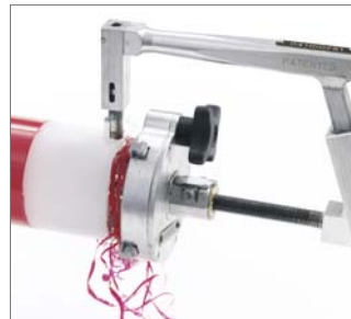
Fig. 93 Scrape the pipes twice.
