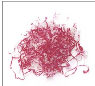
Fig. 112 Scraping should produce a long chip with a uniform thickness (0.1 to 0.2 mm); if required, replace the rotary scraper or knife.
