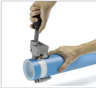
Fig. 42 4. Marking the pipe is unimportant when using a rotary scraper. But only scrape a single layer!
