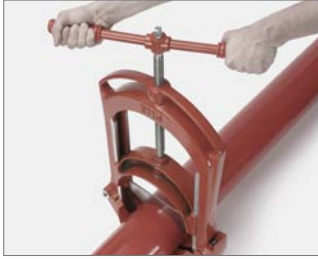
Fig. 25 1. Using a guillotine, trim the pipe at a right angle to the desired length.
