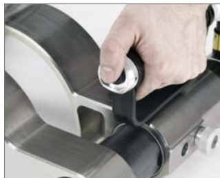
Fig. 34 9. Press the pushbutton on the master cylinder to push the compression sleeve fully into place up to its fitting collar. If required, alter the positions of the pushpins on the movable jaw to ensure the compression sleeve is pushed fully into place. Once completed, pressure and temperature can be immediately applied to the joint.
