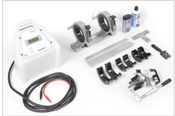
Fig. 85 Tools for creating joints
