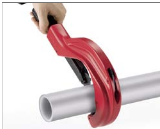
Fig. 17 1. Trim the pipe to the desired length, burr-free and at a right angle.
