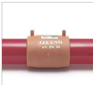
Fig. 108 Using a marker pen, note your personal ID no. and the current date on the electrofusion fitting.
