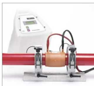
Fig. 115 Scraped pipe ends should be welded as quickly as possible.
