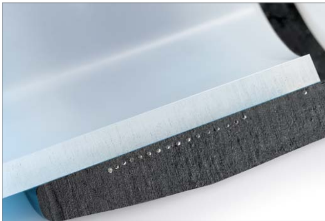
Fig. 36 Integrated resistance wires
