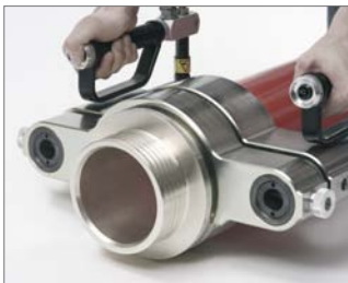
Fig. 33 8. Apply the RAUTOOL G1 125160 compression tool fully. Do not tilt the tool! The tool's entire face must sit flush against and be perpendicular to the connection.
