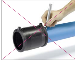
Fig. 66 Do not use the fittings as a marking aid.
