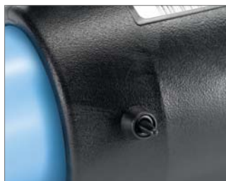
Fig. 78 When welded in place, the indicator nipples at either end of the electrofusion fitting are raised.
