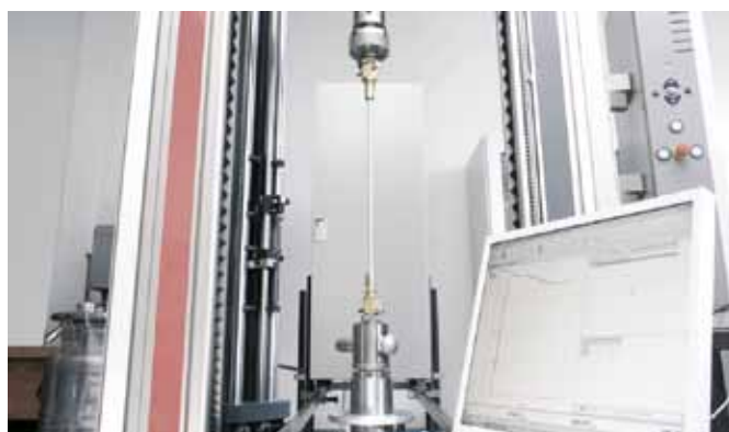
Proceeding a tension test with compression sleeve joint
