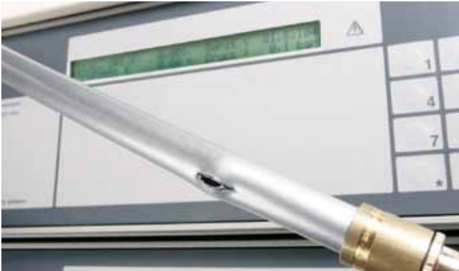
Results of a burst pressure test with the universal RAUTITAN PN20 pipe
