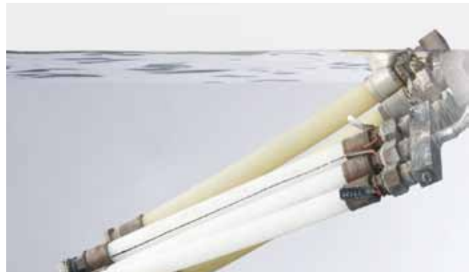
Pipes in a long-term (under 10 bar pressure in a 95°C water bath)
