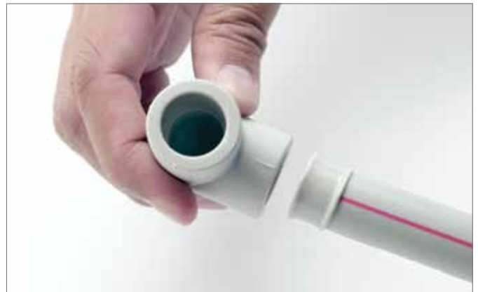
Fig. 8-7 Align the pipe and fitting
