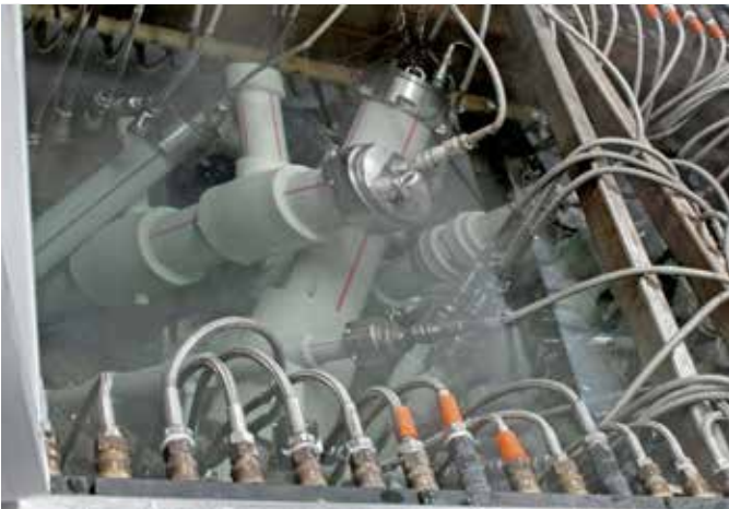
Fig. 3-2 Internal pressure resistance test
