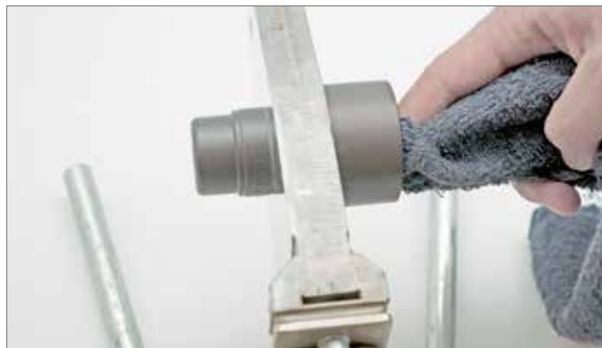
Fig. 8-3 Clean the heating bushes
