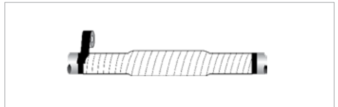
Fig. A1-8 Wrapping the protection area with black/grey tape
