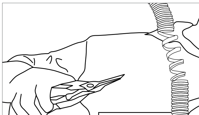
Fig. A2-5 Cutting of RAUGUARD
