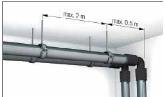
Fig. 7-8 Maximum pipe clamp intervals
