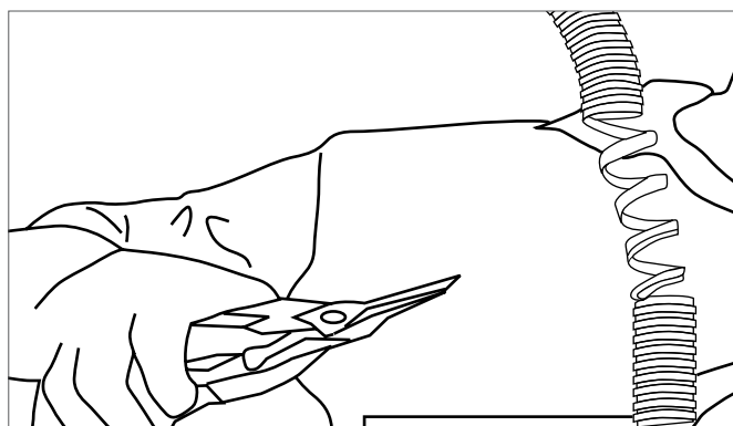
Fig. A2-5 Cutting of RAUGUARD
