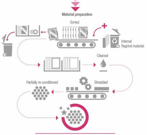
Re-use of recycled material in the inner core of new window profiles through co-extrusion
