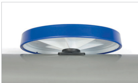
Figure 29: Bottom view of installed disc aerator (disc aerator lower rim touches top of the grommet) 图 29: 安装好的曝气盘底部 (曝气盘的底部与双承接头的顶部接触)
