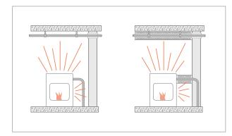
Fig. 6-9 Protection against temperature-induced stress
