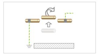
Fig. 6-11 Potential equalisation while replacing pipes
