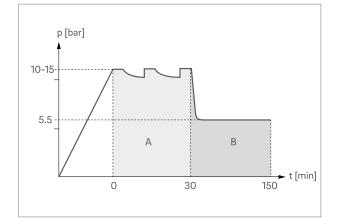
Fig. 7-3 Pressure test diagram
