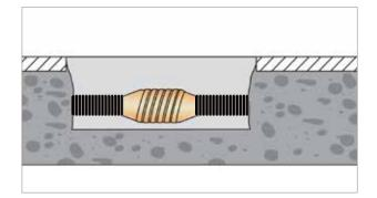
Fig. 6-7 Installation of  $\mathsf{PINC}^{\mathsf{\tiny TM}}$  system within concrete/screed floor with corrosion protection system
