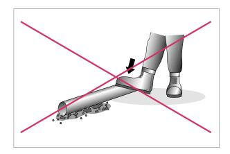
Fig. 4-2 Do not store pipes on sharp-edged surfaces
