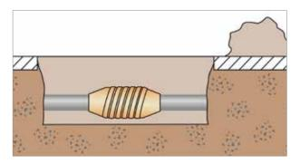
Fig. 6-8 Installation of RAUTITAN system below ground with PINC™ fittings wrapped with corrosion protection system
