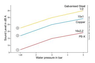
Fig. 7-2 Result of acoustics report from Acoustics Division of the Fraunhofer Institute of Structural Physics
