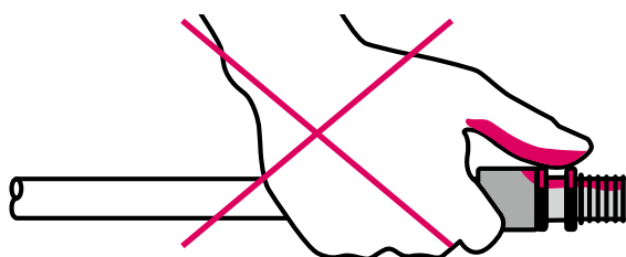
Fig. 41-32 RAUTITAN PX: Avoid unintentional contact with aggressive substances
