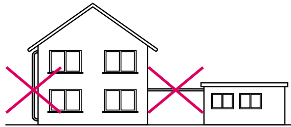
Fig. 31-4 Outside laying is not allowed
