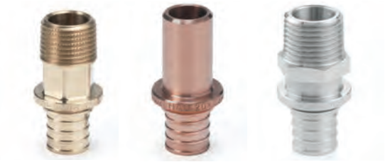
RAUTITAN LX (standard brass), RAUTITAN RX+ (gunmetal) and RAUTITAN SX (stainless steel) fittings
