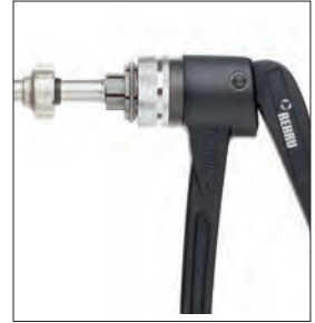
Fig. 14-7 Expand the pipe end once
