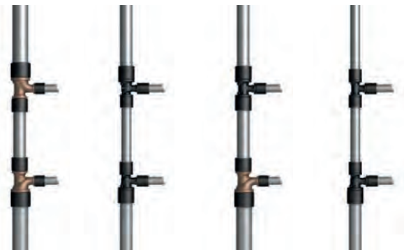
Fig. 05-6 Possible connections of the ring pipe
