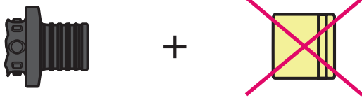
Fig. 36-1 Unapproved combination RAUTITAN PX fitting with brass compression sleeves
