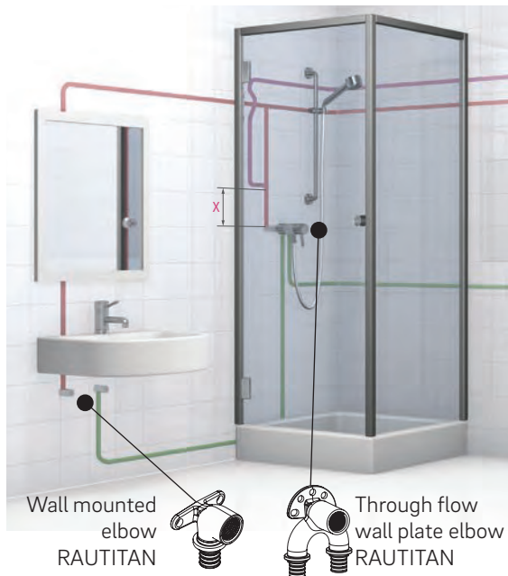
Fig. 05-4 Connection of mixer taps to pipe continuously provided with warm water - Example: Connection from top
