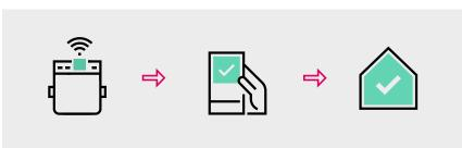
RE.GUARD detects leaks and burst pipes, as well as monitoring appliances using water sensors. If leaks are detected, RE.GUARD shuts off the water supply and alerts you via the app. Costly water damage, mould or time-consuming hassle with insurers can be easily prevented.
